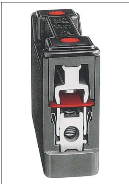
Cut-away view of 63 amp front connected contact assembly
